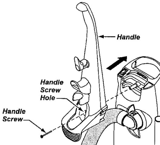
Begin to tighten the screw with your fingers. It may be necessary to adjust the handle slightly.
